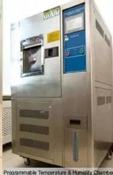
Programmable Temperature & Humidity Chamber
