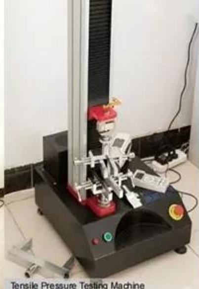
Tensile Pressure Testing Machine
