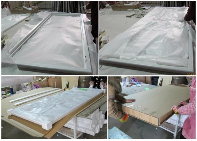
**B.**For shutters with more than two panels, panels and frames packaged seperately.
