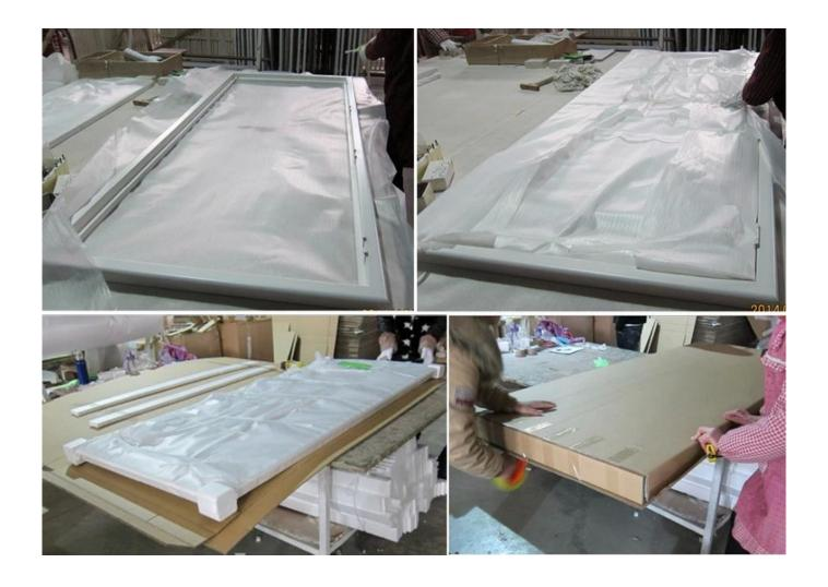
${f B.}$  For shutters with more than two panels, panels and frames packaged seperately.
