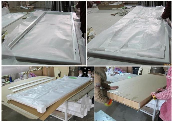
${\bf B}. {\bf For}$  shutters with more than two panels, panels and frames packaged seperately.
