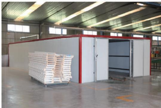
In order to ensure that our products can maintain excellent quality in various environments, we have specially added a greenhouse test link for our products. The greenhouse simulates different temperature and humidity conditions, giving us insights into how the product will perform under various extreme conditions.
