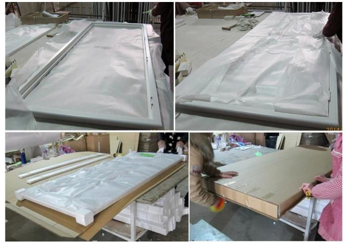
$\boldsymbol{B}. For hatches with more than two panels, panels and frames packed separately.$
